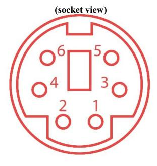
**6 pin Mini DIN jack:** A straight 6 pin Mini Din cable can be used to connect WolphiLink to an FT817 transceiver. Other radios might need a custom made cable.
